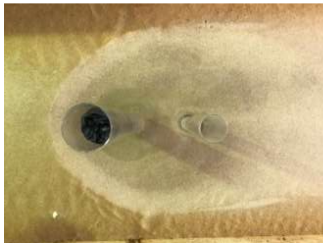
Figure 7. Scour after 144 hours
