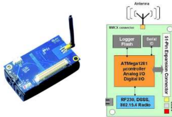
Figure 4. IRIS XM2110 system and its block diagrams
