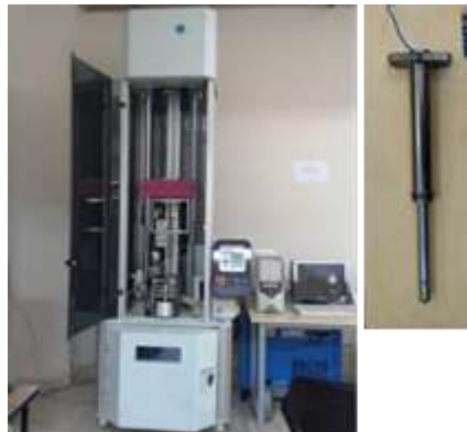
Figure 4. Low velocity impact testing machine and impactor
