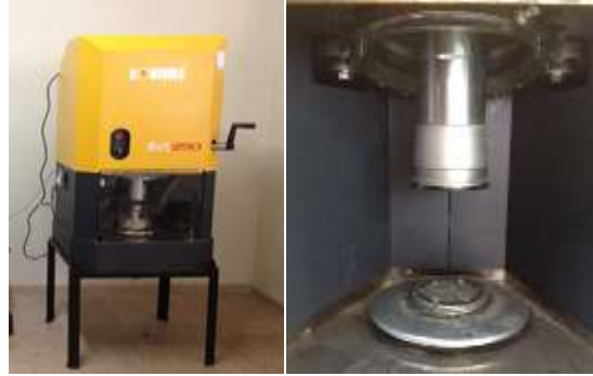
Figure 2. Gyrotory press and compression head.
