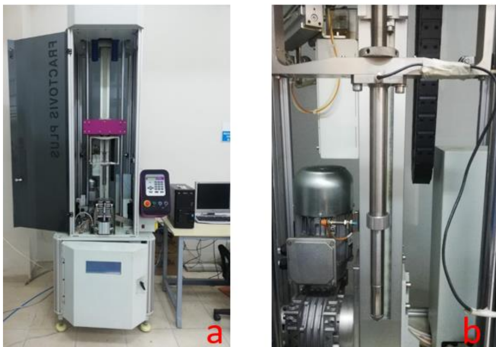
Figure 4. a) CEAST-Fractovis Plus impact testing machine, b) Impactor
