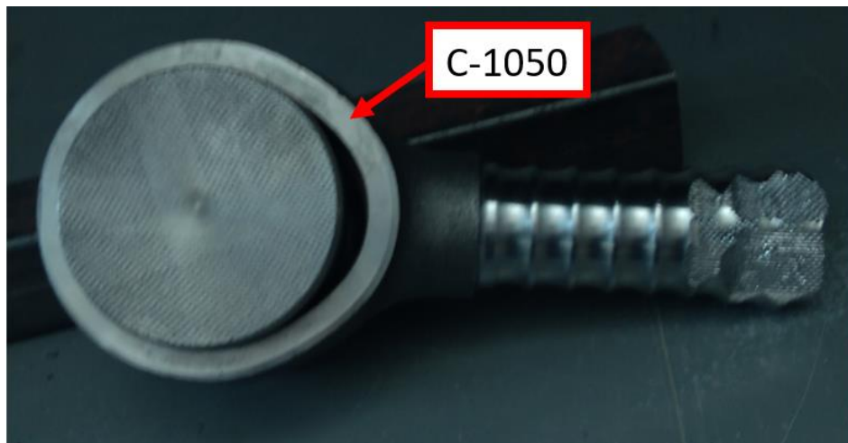
Figure 6. Test specimen after the tensile test
