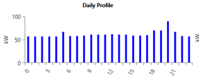
Figure 2. Daily load curve of the village
