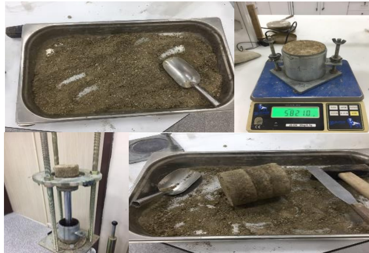
Figure 2. Sample preparation of compaction test
