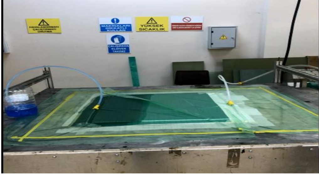
Figure 1. Production of sandwich composite by vacuum assisted resin infusion method
