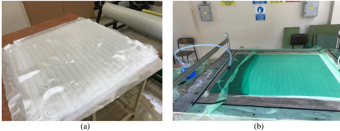
Figure 1. (a) Preparing of S2 Glass Fibers, (b) Composite manufacturing system
